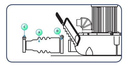
Use the flexible inlet connector (A) for side inlet connections. Using a metalwork saw, saw off the desired inlet point, remove any burrs and then fix the flexible inlet connector with the hose clip (D).
