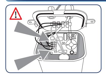
There is the option of connecting an alarm (light, bell) on to the electronic circuit board (2 terminals fed with 220V). If the motor is run continuously (more than 5 minutes), the contact will be made. This enables the user to carry out a check if he wishes.
