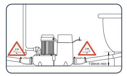
To connect a bathtub (or shower), make sure the waste trap height is raised by at least 15cm above floor level.
