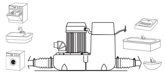
Sanicom is a lifting pump for wastewater used in commercial applications (restaurants, hairdressing salons, the catering industry etc.). The unit operates automatically, has a high performance level, and is safe and reliable, provided all the rules for installation and maintenance in this notice are strictly followed. Especially those indicated by:
