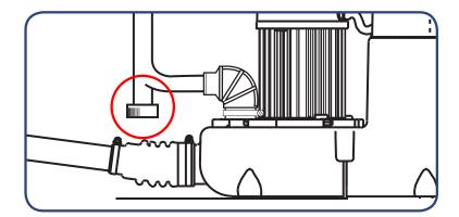
Allow for a drain-off point at the bottom of the rising discharge pipe. Ensure that the unit is easily accessible for possible maintenance.
