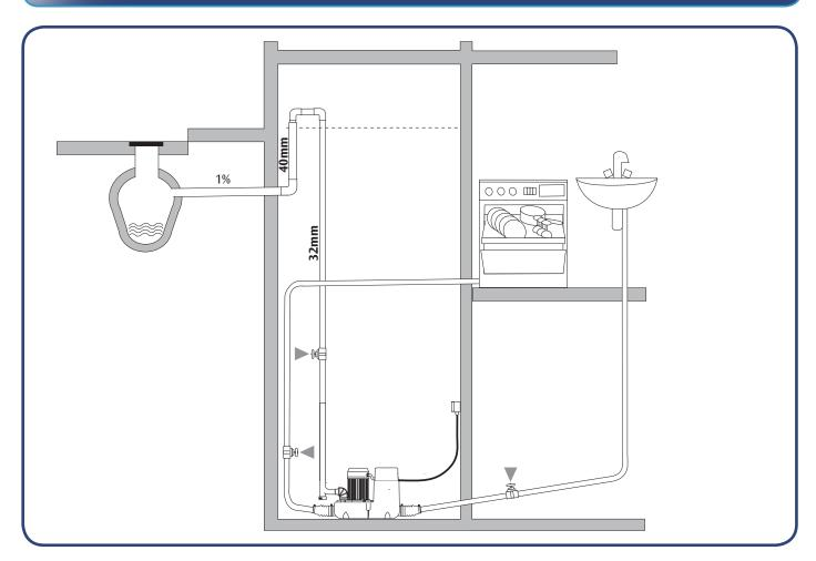
The disposal of waste from the Sanicom can discharged through a 32mm diameter copper or plastic pipes (or PVC, ABS, etc.).
