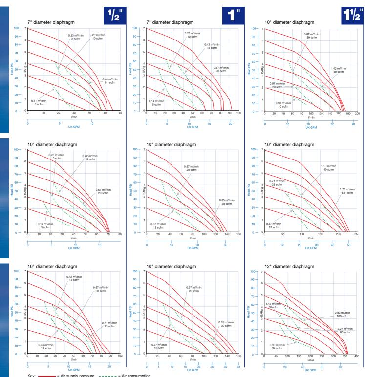
To view these flow rates in greater detail, go to www.flotronicpumps.co.uk/flowcurves
