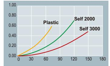
l/min. Thanks to the reduced force necessary to open the valve, the Self 3000 nozzle can be used for the transfer of oil with working pressures up to 10 bars (142 psi). **Plastic** versions with a flow rate up to 80 l/min are also available.
